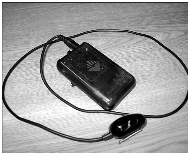
Tiny and unobtrusive, the microphone and transmitter components of the Phonic Ear sound field system measure just inches across, but deliver remarkable clarity.
